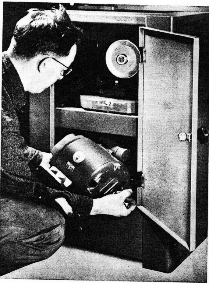
Fig. 5. Installing the Motor.
