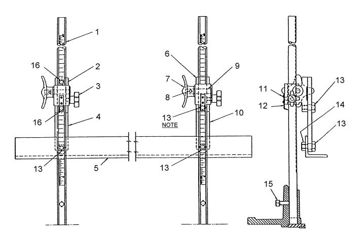
$\underline{\mathsf{NOTE:}}$  R.H. LINK (10) IS ASSEMBLED TO R.H. GAUGE HOLDER (6) WITH ONE PIVOT STUD (13) TO PROVIDE FOR ANGULAR SETTING OF BACKGAUGE.
