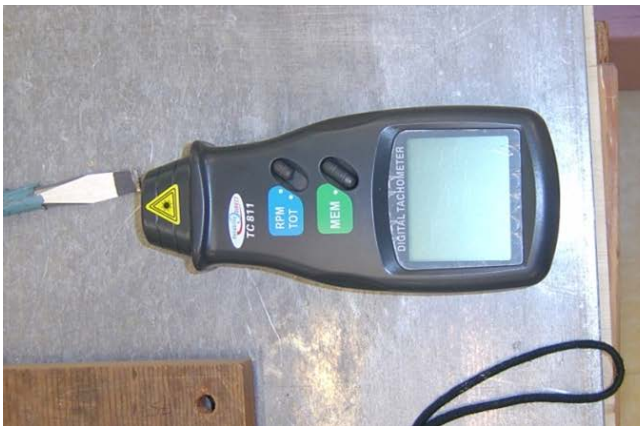
Tachometer - measures the speed of the rotor
