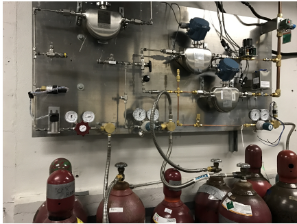
Figure 2: Intake flow meter, pressure gauge and sensor mounting wall.
