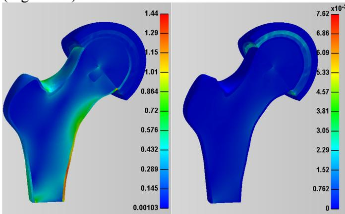
**Figure 4: A (left). Effective stress distribution. B (right). Effective strain distribution.**
