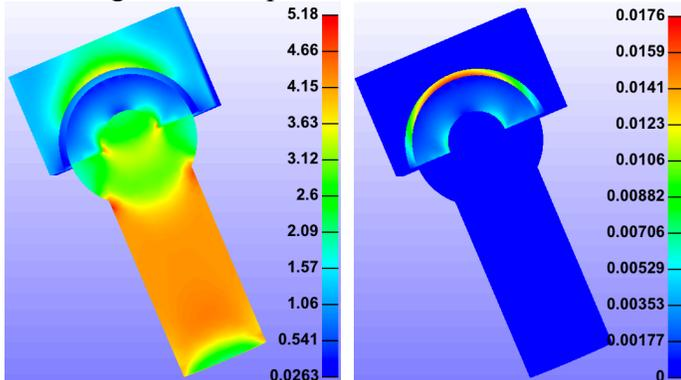
**Figure 3: A (left). Effective stress distribution. B (right). Effective strain distribution.**
