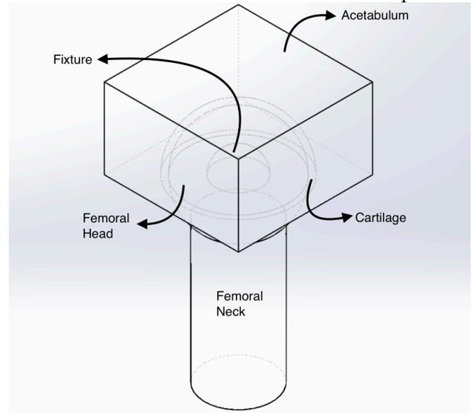
**Figure 1: Model 1 geometry**
