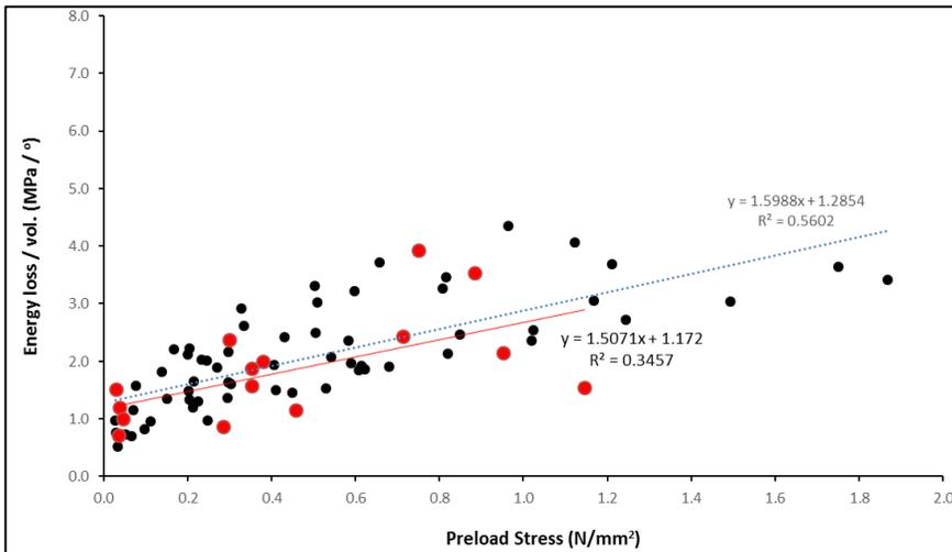
Fig.2: Sample results showing hysteresis energy loss/volume vs. preload stress. Injured samples are plotted in red, healthy samples in black. There is no change with injury.
