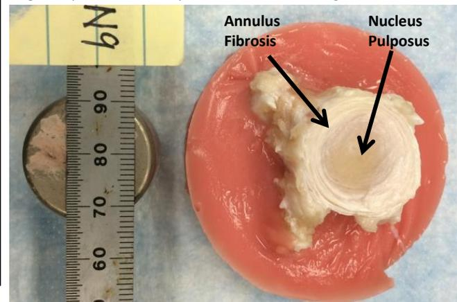
Fig.4: Cut disc with scale for reference
