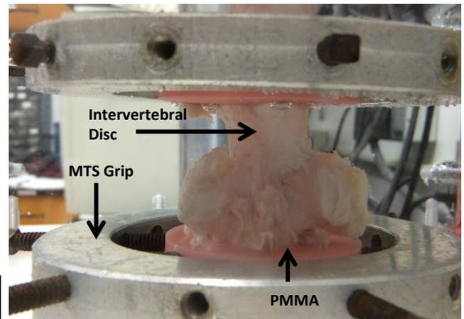
Fig.3: Experimental setup for mechanical testing with MTS
