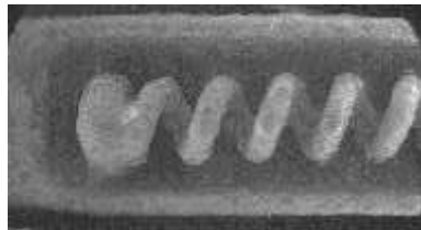
Figure[2]: 3D printed Spring Diode in SEM
