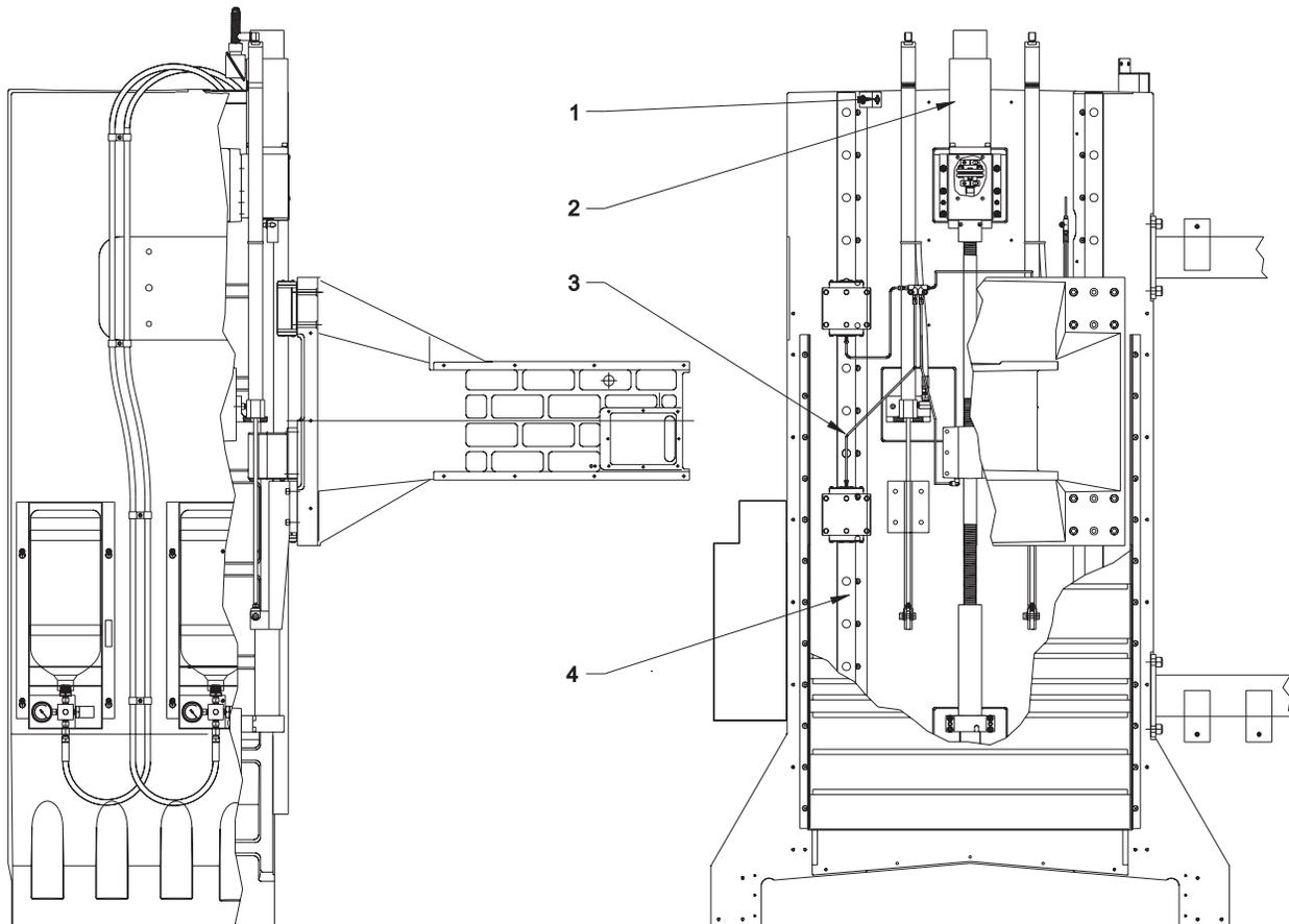
1. 32-2050 Telemechanique limit switch assembly
