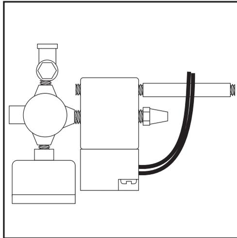
Figure 4.1-5 Top view of spindle lube/air solenoid assembly.
