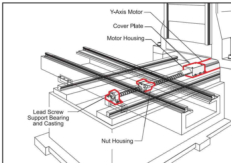
Figure 3.9-5 Y-axis lead screw and components.
