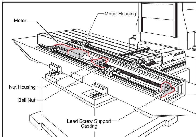
Figure 39-1. X-axis lead screw and components.
