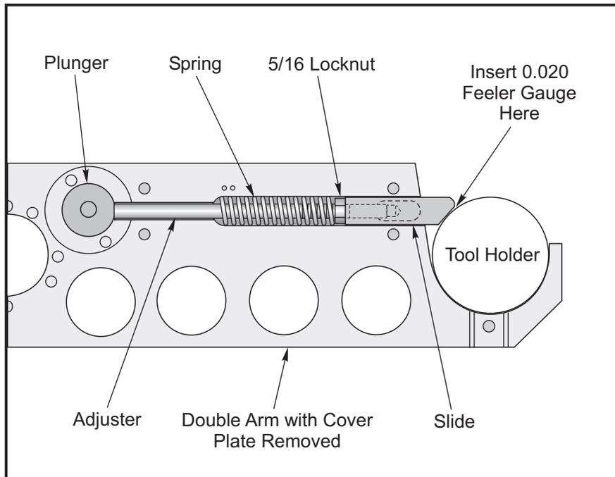
The plunger will not return reliably to the fully raised locked position when the tool is inserted, if there is insufficient clearance. The toolholder will be excessively loose in the doublearm if there is too much clearance.
