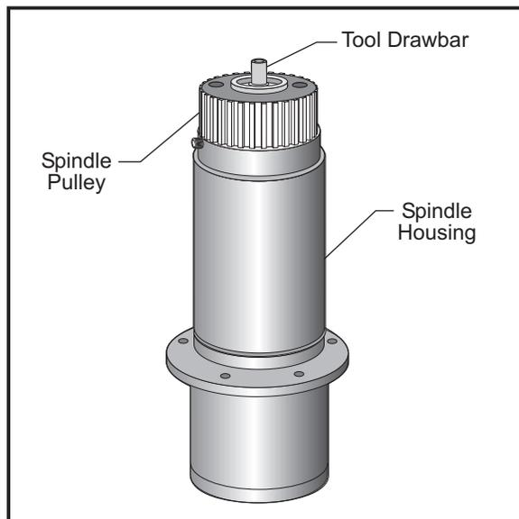
Figure 3.4-2. Spindle cartridge.
