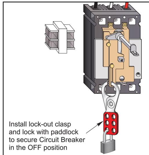
Make sure the circuit breaker is locked in the off position before attempting any electrical work to avoid possible shock.
