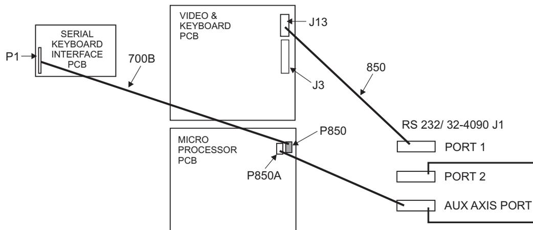
\* Serial interface replaces cable 700 with cable 700B.
