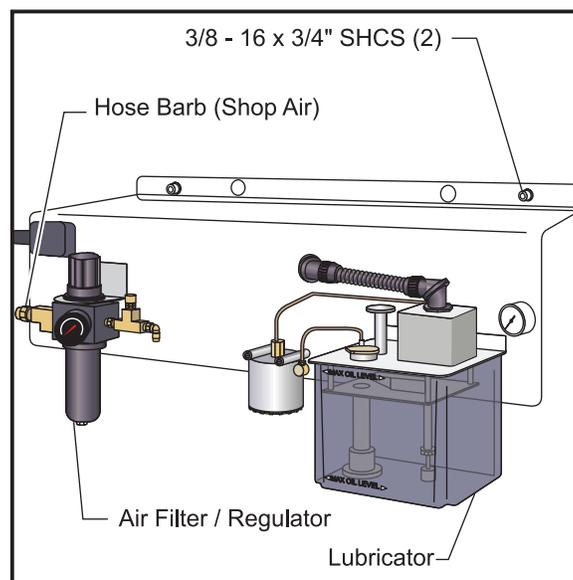
Figure 3.8-4 Lube/Air Panel.
