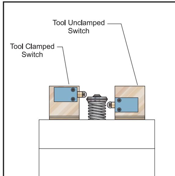
Figure 3.2-12 Tool Clamp / Unclamp Switches.
