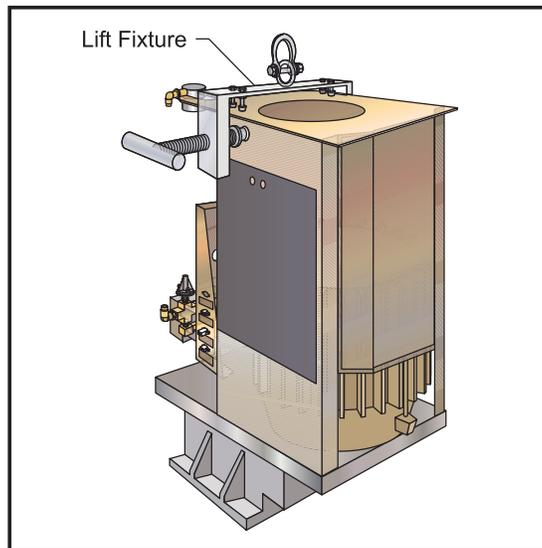
Figure 3.7-10 Lifting position for VF-1 through 4.
