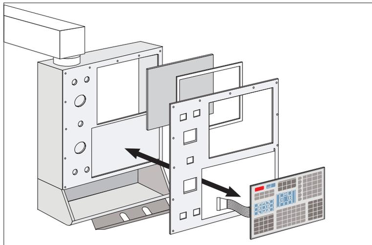
Figure 4.5-5. Keypad installation.
