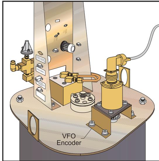
Figure 4.6-2 Encoder installation for direct drive machines
