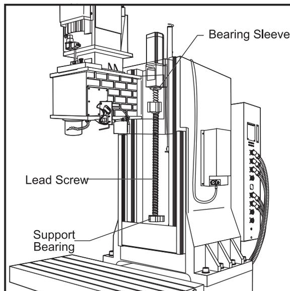
Figure 3.10-3 Z-axis bearing sleeve.
