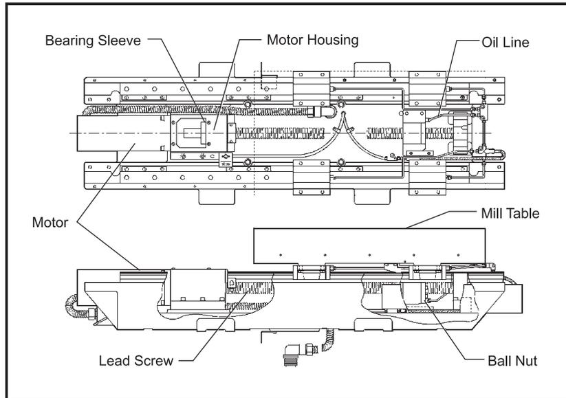
Figure 3.9-2 Lead screw assembly.
