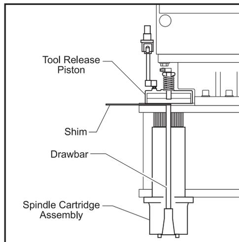
Figure 3.2-7 Placement of shim before checking switch adjustment.
