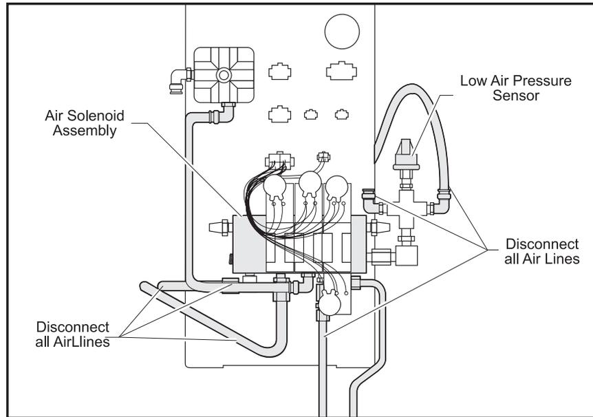
Figure 4.1-1 Air solenoid assembly.
