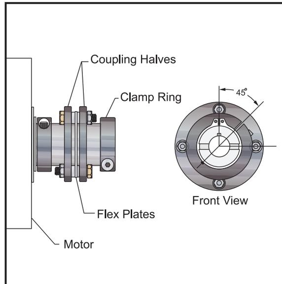
Figure 3.8-2 Motor coupling components.
