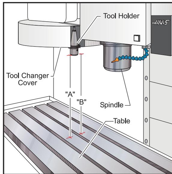
Figure 3.6-1 Checking tool offset reference.
