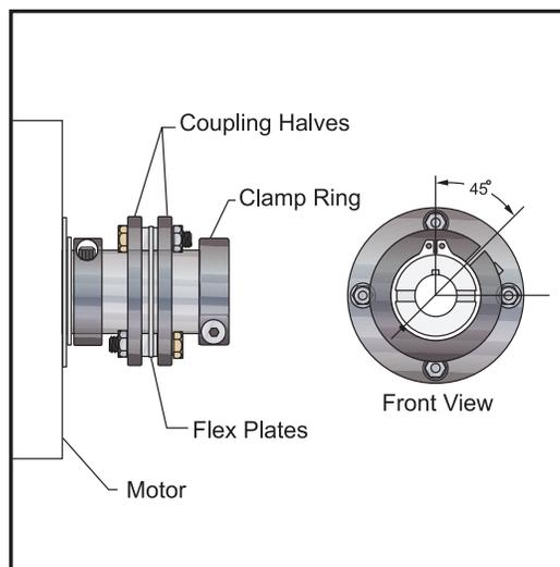
Figure 3.8-7 Motor coupling.
