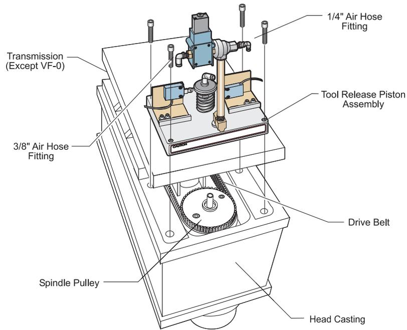
Figure 3.3-2 Mounting location for tool release piston assembly
