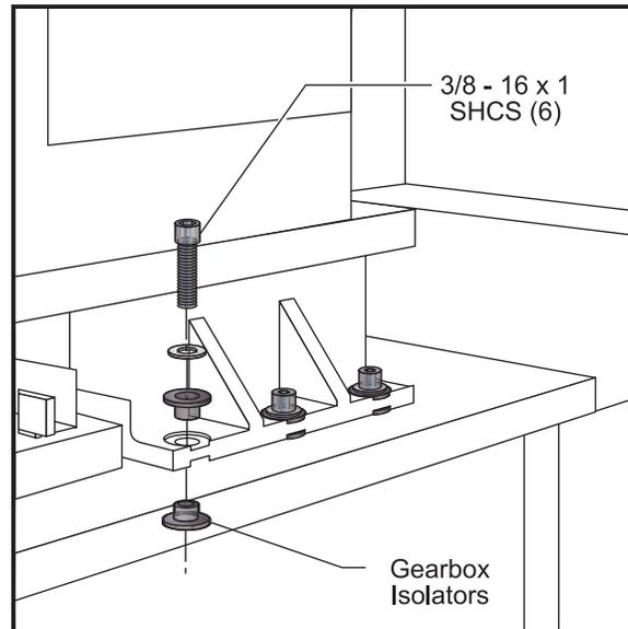
Figure 3.7-11 Gearbox isolators.
