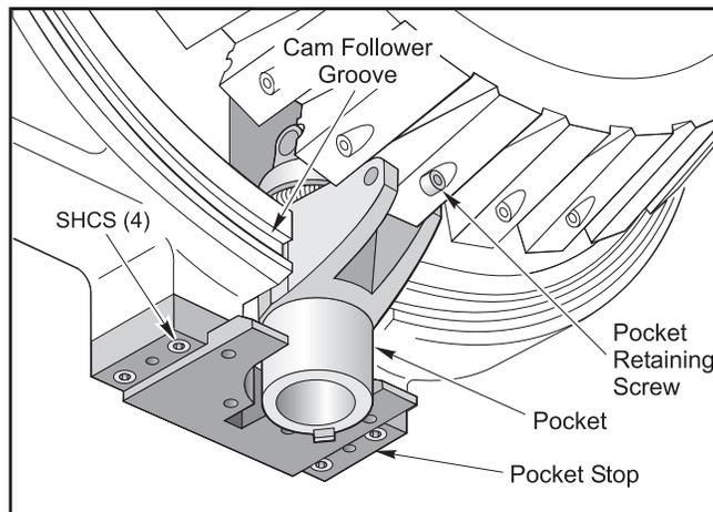
**NOTE:** Do not remove the set screws. Doing so will change the pocket slide and groove alignments.
