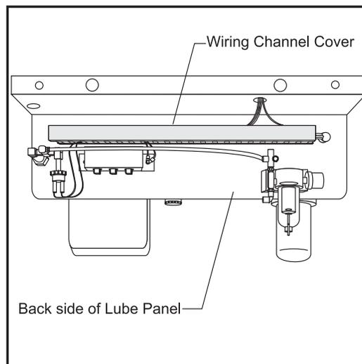
Figure 4.1-4 Top view of spindle lube/air solenoid assembly.
