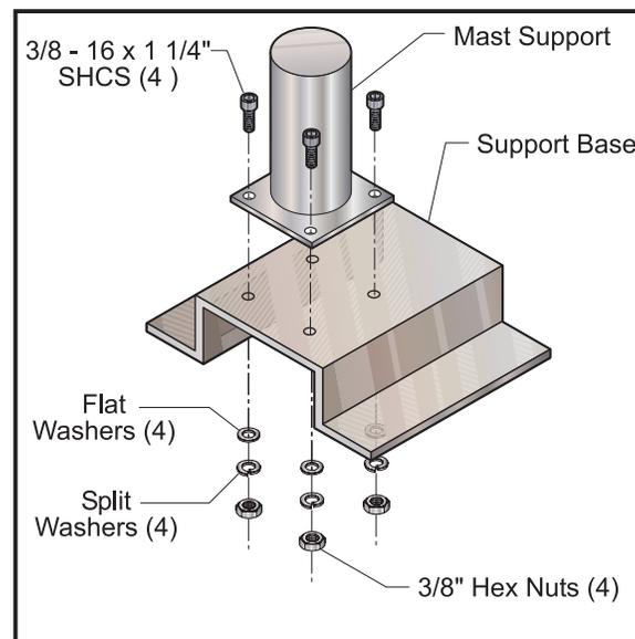
Figure 3.7-3 Exploded view of boom modification plate components.
