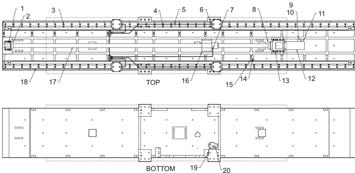
1. 20-0152 Bearing housing 40mm and 50mm ballscrew
