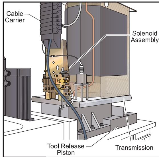
Figure 3.7-6 Solenoid bracket with all lines connected.
