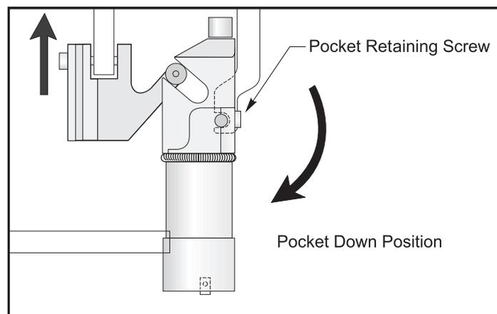
6. Remove the tool changer pocket by carefully maneuvering the pocket out of the carousel, taking care not to drop the pocket slide.
