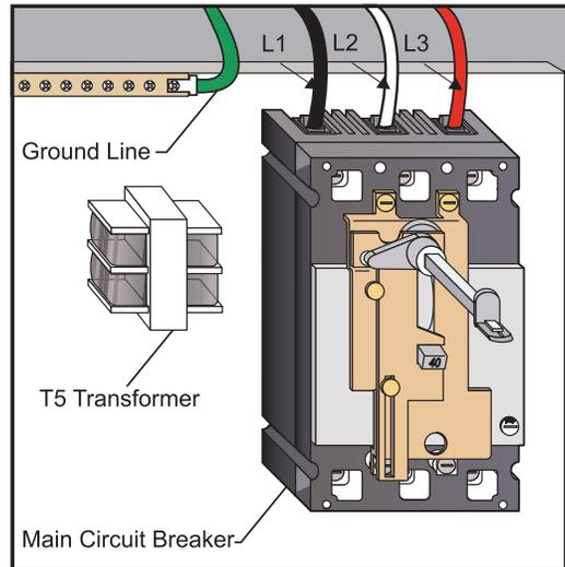
1. Hook up the three power lines to the terminals on top of the main switch at upper right of electrical panel and the separate ground line to the ground bus to the left of the terminals.
