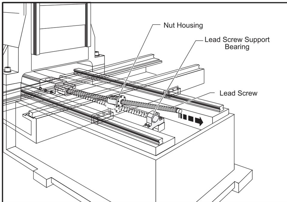
Figure 3.9-6 Pull lead screw forward around bearing support,...
