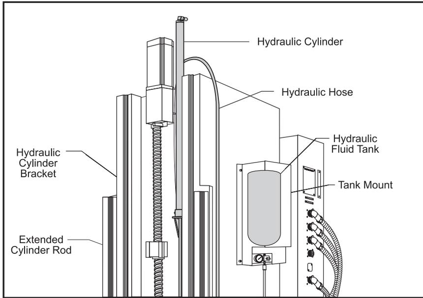
Figure 3.14-4 VF-Series hydraulic counterbalance - right side view.
