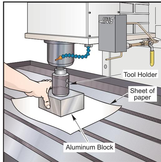
Figure 3.2-9 Pushout Adjustment.
