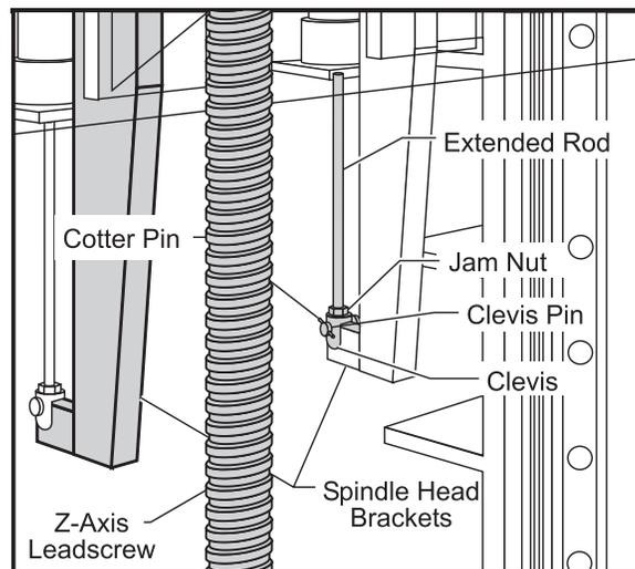
Figure 3.14-3 Hydraulic Cylinder Rod Installation for VF-1 through 4 and (VF-6/8).
