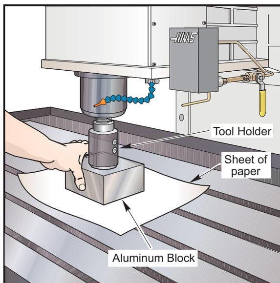
Figure 3.2-4 Placement of aluminum block under spindle.
