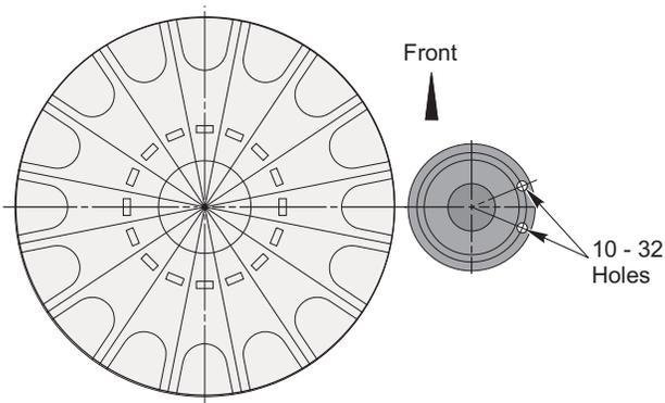
Figure 3.4-3 Underside view of spindle cartridge.
