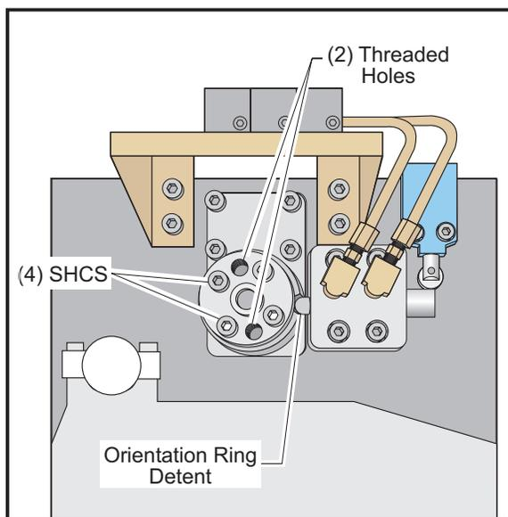
Figure 3.5-1 Top view of spindle orientation components.
