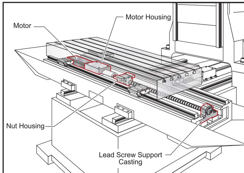
Figure 3.8-1 X-axis motor and components.
