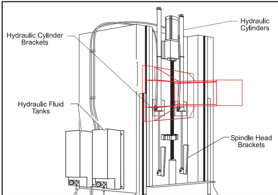
Fig. 3.14-5 VF-Series hydraulic counterbalance view - left side view.
