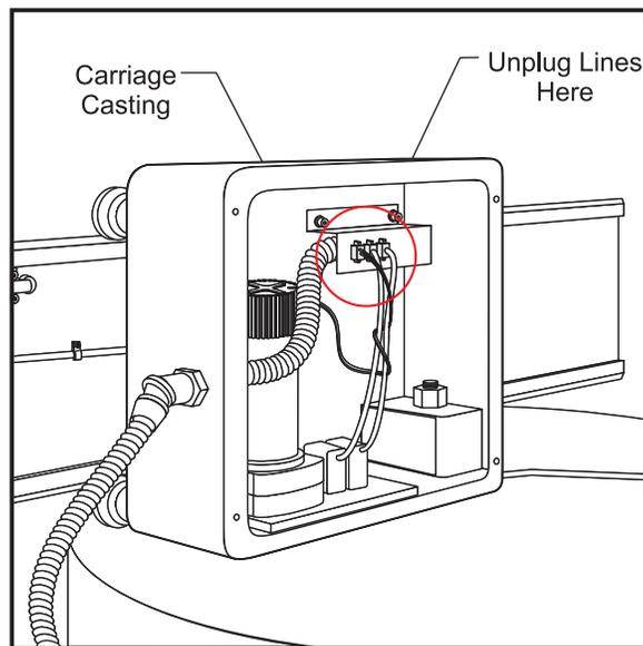
Figure 3.11-6 Carriage casting with cover removed.
