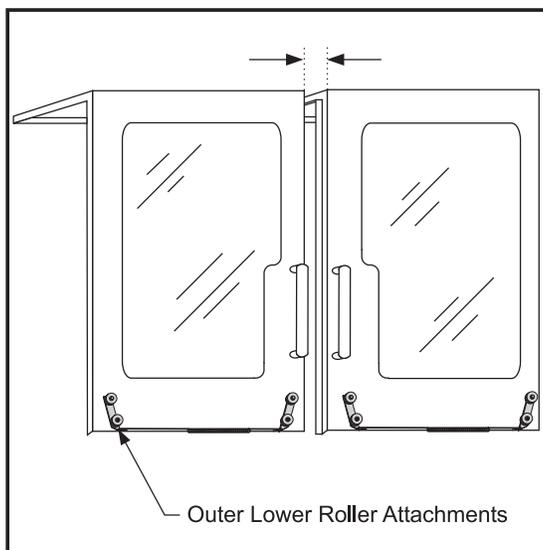
Figure 3.13-2 View of vertical gap between front doors.
