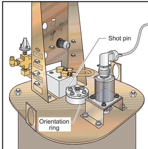
Figure 3.5-2 Direct drive motor with orient ring location.
