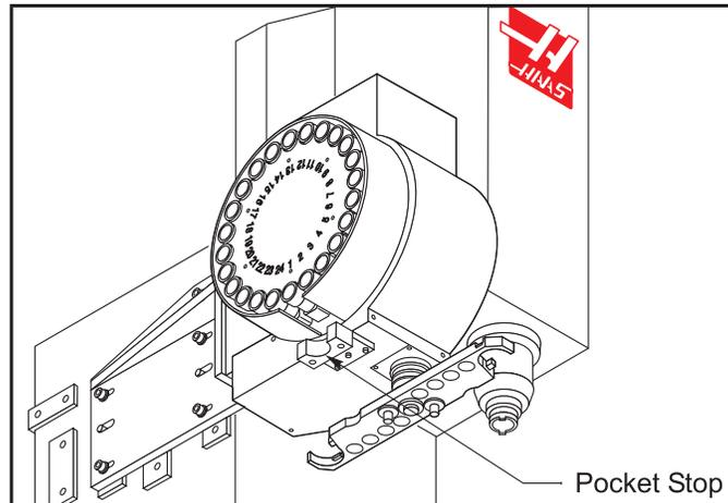
4. Remove the shoulder bolt from the back of the pocket slide.
