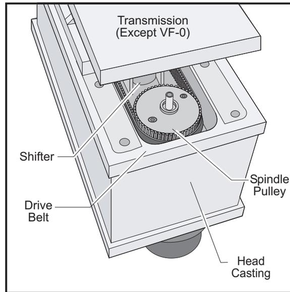
Figure 3.3-2 Head casting area showing belt location.
