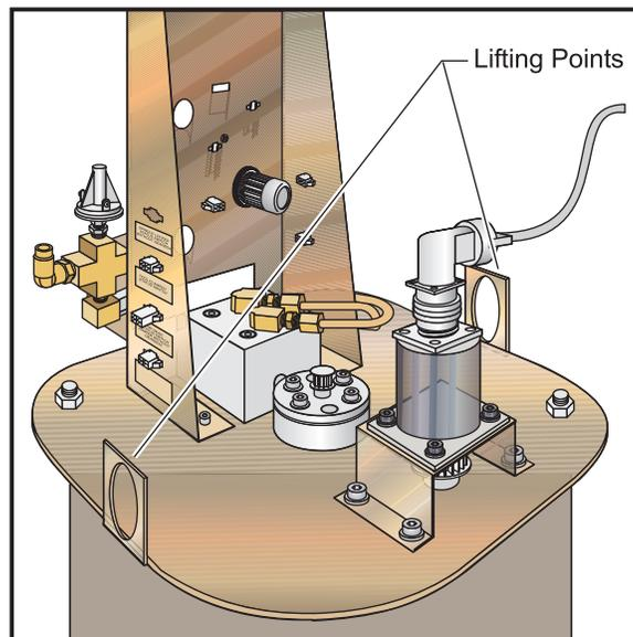
Figure 3.7-1 Direct Drive with lifting eyeholes.
