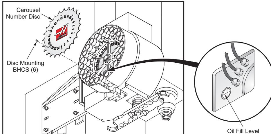
The SMTC is factory filled with the appropriate level of oil and does not need to be changed under normal conditions. As a precaution, check the oil level annually. Oil will not need to be added as long as the level remains viewable in the sight glass as shown above. Should the level drop below the sight glass, call the HAAS service department.
