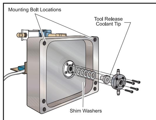
Figure 3.2-5 Tool release piston assembly (TSC shown).
