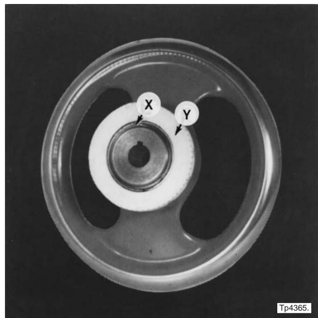
Figure 1.39 - Carriage Handwheel and Dial
