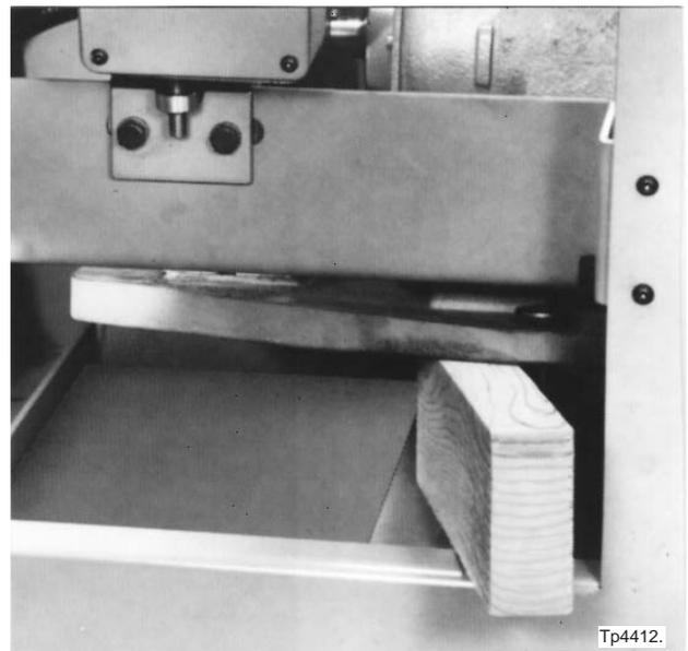
Figure 3.6 - Motor Mounting Plate Blocked in Position
