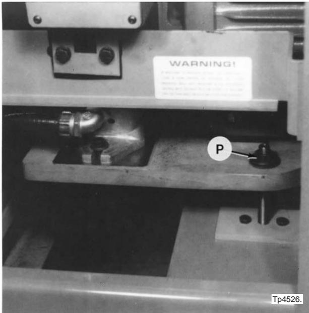
Figure 4.70 - Drive Belt Adjustment Screw
