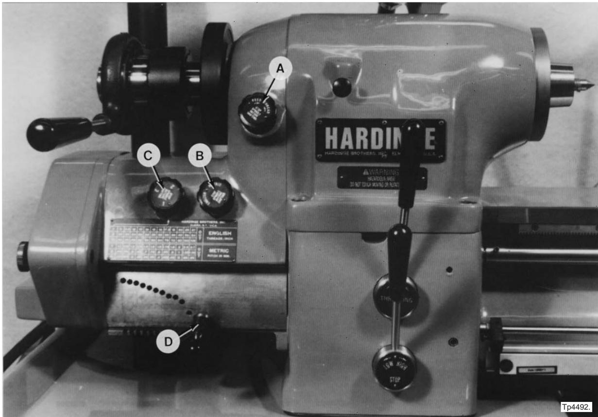
Figure 4.36 - Gearbox (Front View)
