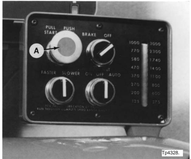
Figure 1.1 - Variable Speed Control Box (HLV®-H Machine Model Shown)
