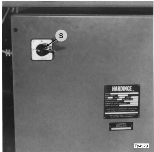
Figure 4.73 - Main Disconnect Switch
