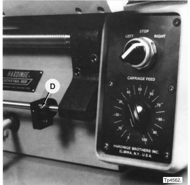
Figure 6.15 - Stop Rod Positive Stop
