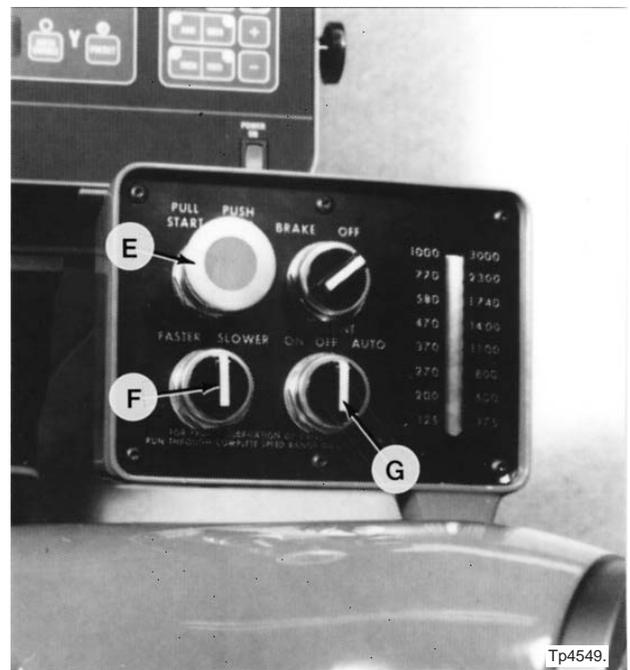
Figure 6.2 - Variable Speed Control Box
