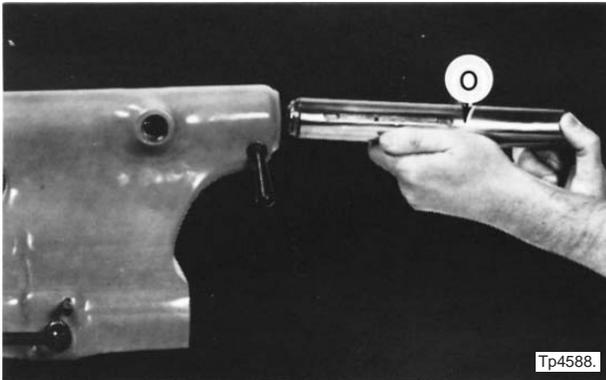
Figure 6.43 - Tailstock Spindle
