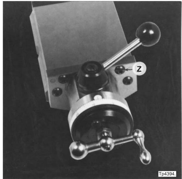
Figure 2.12 - Tool Post Slide
