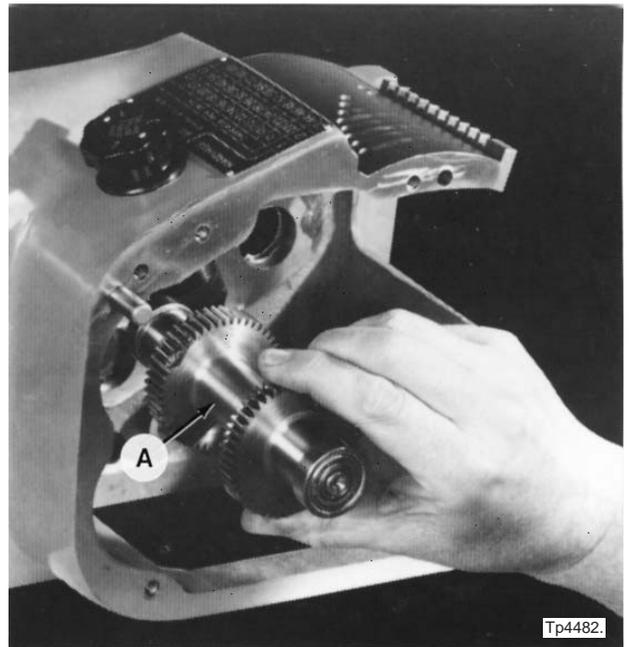
Figure 4.26 - Reverse Shaft Removal
