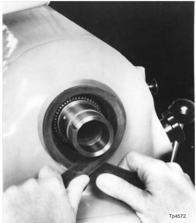
Figure 6.26 - Spindle Belt Replacement
