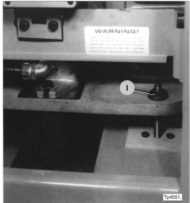
Figure 6.4 - Drive Belt Adjusting Screw
